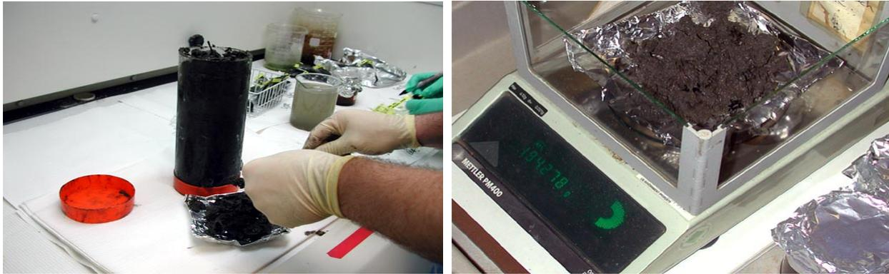
Figure 9. Removing and weighing sediment
