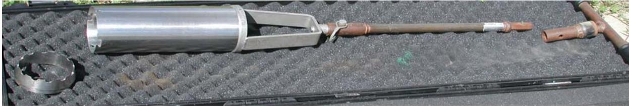
Figure 7. Sediment coring device
